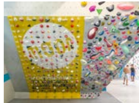
Hybrid system board comprising synthetic resin holds with a software-based diode system on the left-hand side (commercially available) and a section without any pre-defined boulders on the right-hand side. Boulderwelt Ost bouldering gym in Munich, Germany.
