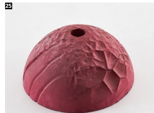
25 Brian Meuse 3D designed and printed the master for this hold, then molded it to make repeatable copies in plastic (USA 2013/2014).
